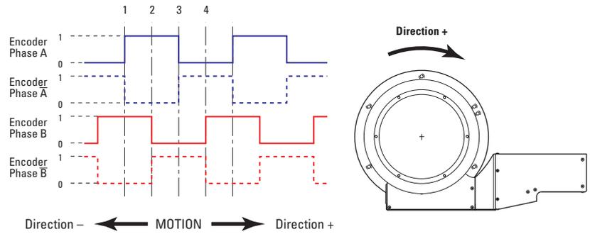
The incremental sensor consists of an optical scale and an encoder head. When the carriages of the stage move, the encoder head generates square signals in quadrature, sent to pins #19, #20, #23 and #24 of the SUB-D25 connector.
