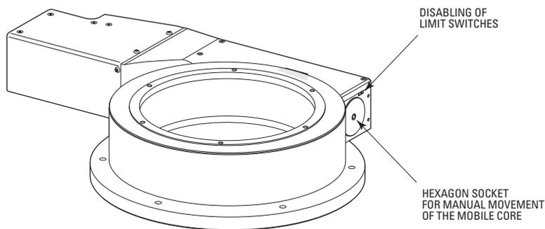
At the end of the drive screw in RV stages (side opposite motor), a hexagon socket is given for manual movement of the mobile core, using an “Allen” wrench.
