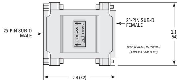
This regulator is available as an option. Please note that for best efficiency, this regulator should be attached to the stage to re-adjust the 5 V coming from the controller through the long cable.
