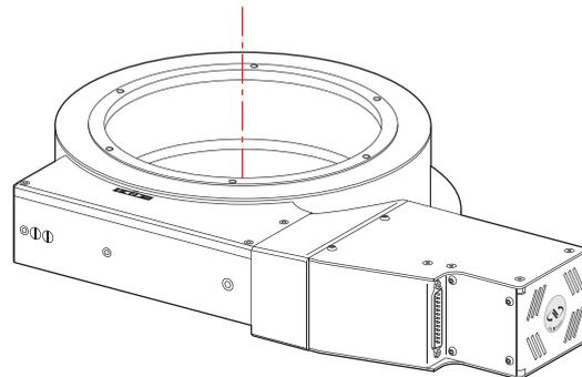
The RV rotation stage is fixed on a horizontal surface. The external flange has various holes provided for fastening.
